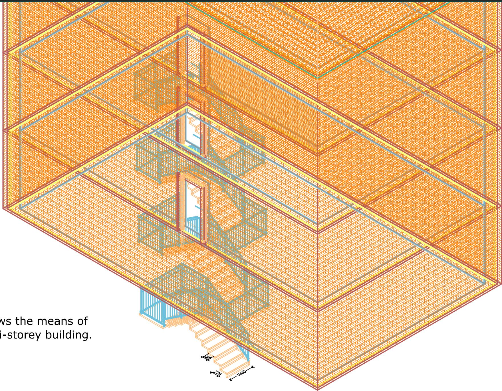
This drawing shows the means of escape for a multi-storey building.
